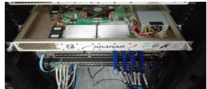
SKARAB Board, for SKA-SA Digital Spectrometer. Image Credit: Peralex, South Africa.
