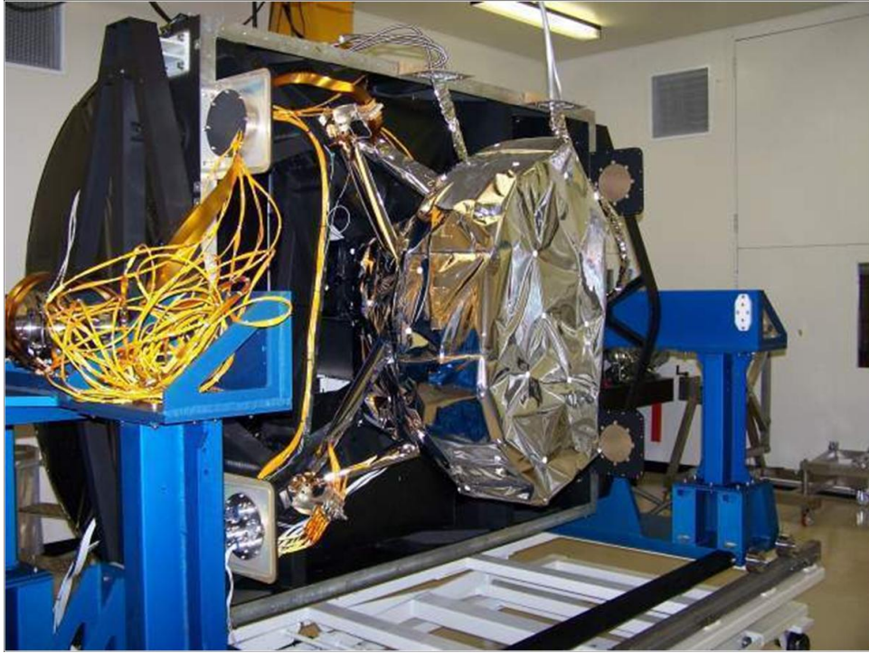
MIRI Verification Model (VM) encased in a Mylar blanket prior to vacuum cryostat testing.
