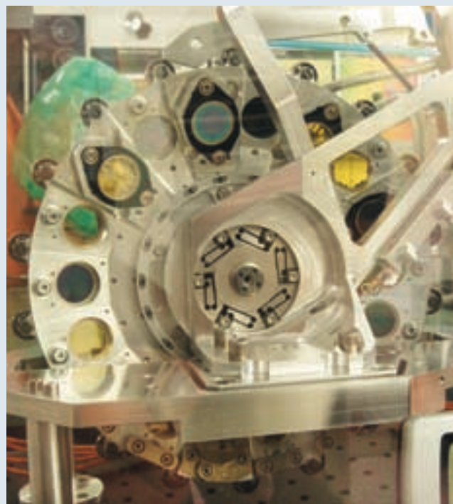
Figure 11: Mid-infrared filters, supplied by the Dublin Institute for Advanced Studies, that were used to populate the MIRI verification model (VM) filter wheel in the CEA, Saclay
