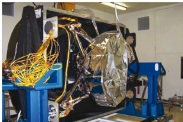
MIRI Verification Model (VM) encased in a Mylar blanket prior to vacuum cryostat testing
