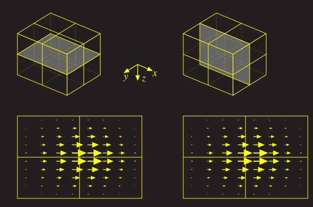
But this gives continuous normal electric field, by construction, even if there's a discontinuity in conductivity.
