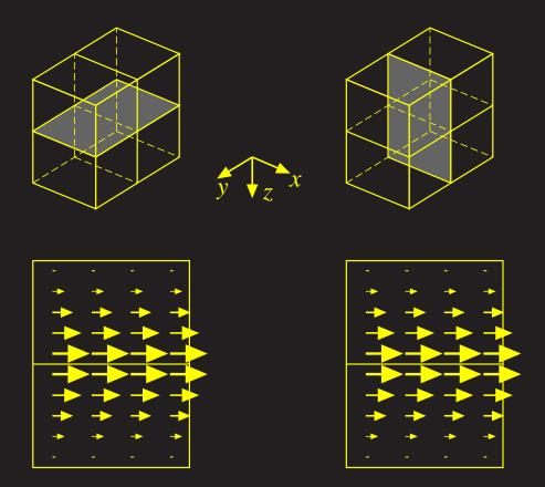
These basis functions can give a discontinuous normal electric field.
