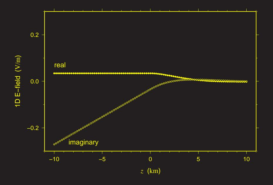
(Homogeneous halfspace of 0.01 S/m; "air" of  $10^{-8} \text{ S/m}$ ; 3 Hz.)
