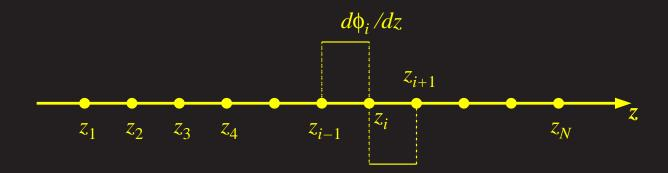
$$\int_{z_i}^{z_{i+1}} \phi_j \, \frac{\partial^2 \phi_i}{\partial z^2} \, dz \, = \, - \int_{z_i}^{z_{i+1}} \frac{\partial \phi_j}{\partial z} \, \frac{\partial \phi_i}{\partial z} \, dz \, + \, \left[ \phi_j \, \frac{\partial \phi_i}{\partial z} \right]_{z_i}^{z_{i+1}}$$
